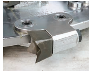
Turn, Sharpen, or Replace Teeth
